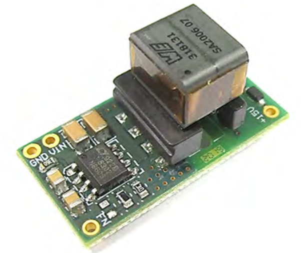
Figure 5 : Würth Elektronik reference design for a compact, isolated DC/DC converter for HV SiC/IGBT Gate Driver.
